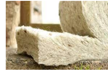
Hemp insulation (Source: Unyte Hemp)
