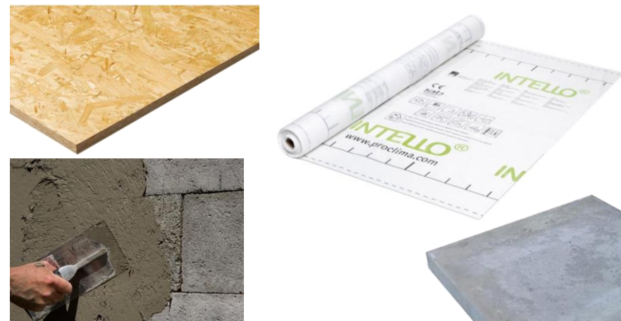
Large airtight surfaces within buildings are typically created from airtight OSB, parge coat and wet plaster applied over blockwork, concrete castings, or specialised airtight membranes. Do not use cheap polythene membranes, as these are fragile and lack the rigidity to tape without creases that cause leaks. (Source: Pro Clima)
